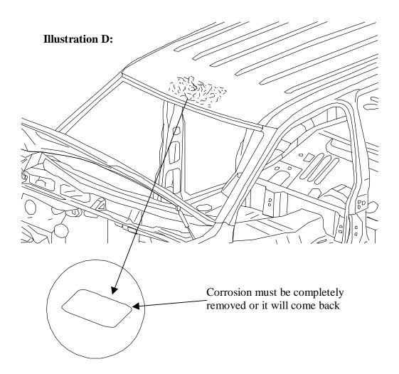
3. All paint, primer, adhesive, and any other protective coatings must be removed from all mating surfaces prior to application of any adhesive for the backer panels. Grind a 2.5cm (1 inch) contact area on all panels where you will do your backer panel bond. The metal should be bare and shiny in appearance. The panels to be used as the backer panels must also be free of all coatings. Bevel the backer panel to prevent moisture or condensation from collecting between the panels.
