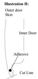
Note: There must be drain holes in the bottom of the door. If you apply adhesive to the bottom of the door make sure to you have a drain hole at the front and rear of the door.
