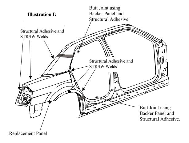
Note: Using the Weld Bond Publication #81-170-03005 make test samples with scrap metal and adhesive to ensure your STRSW welder is ready to apply welds as required.
