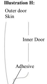
Note: There must be drain holes in the bottom of the door. If you apply adhesive to the bottom of the door make sure to you have a drain hole at the front and rear of the door.
